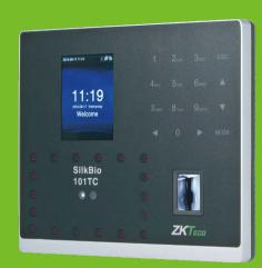
SilkBio-101TC is Time & Attendance and Access Control Terminal to be associated with SilkID fingerprint reader, face recognition and RFID card functions. With the new SilkID fingerprint reader, the operation remains stable under strong light source and high preciseness of verification of wet and rough fingers. With latest facial algorithm and the innovation features, SilkBio-101TC is bringing you the whole new experience.
